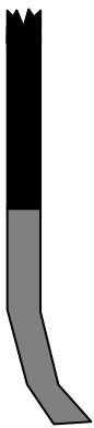
Figure 19: Open face can be achieved by bending the lower part of the blade forward.
